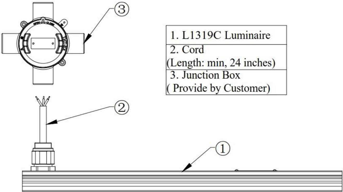
1. For luminaire model with suffix "WHT Mounting": Insert the cord (2) through the conduit (not shown, provide in the field) into the Junction Box (3) (provide in the field).
